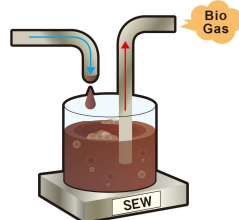
BIO GAS GENERATOR
